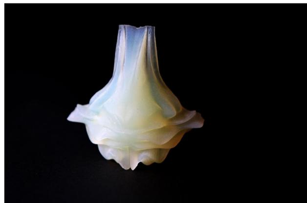
Figure 8 | Nose project *Radiator / resonator* – photo of 3D printed object in Flexible material Tango Plus 9740. Technology polyjet, solidified liquid photopolymer by using UV light (front view).
