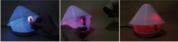
Figure 1 | Shybo robot. From left: colour selection in train mode; sound recording in train mode; scared status in play mode.
