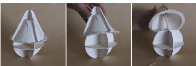
Figure 7 | Second paper prototype. The hat has the shape of a cone, rounded on top. The two elements are joint by providing the hat with two axes joint to the structure of the body through a pivot.
